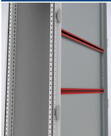
**Description** The MPR and MPWR reinforcement kits stiffen the mounting plate and allow heavy components to be mounted while dampening down any vibrations. The MPR suits standard mounting plates (as supplied with the enclosure), while the MPWR suits the optional MPW wide mounting plate. Supplied as a kit of two profiles with mounting accessories It is recommended for use with mounting plates wider than 1000mm. The profiles should be equally spaced on the rear of the mounting plate.
