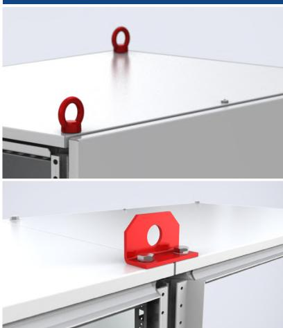
**Description** LE lifting eye bolts mount directly to the enclosure corners for when lifting operations are required. Complies with DIN 580 lifting requirements. M12 thread. 3400N per lifting eye with max angle of 45°. The LE9304 may be used to lift individual enclosures or to lift bayed enclosures in conjunction with the LC lifting device.
