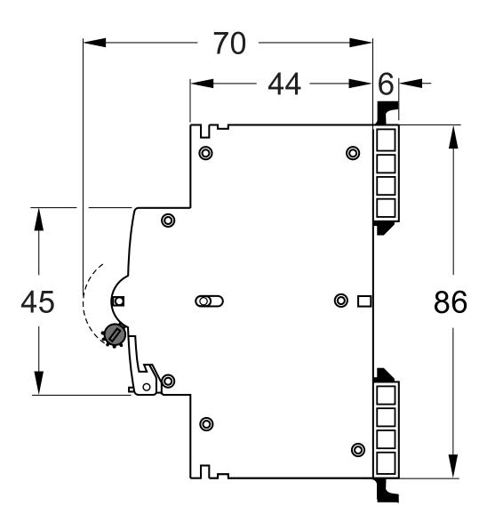
NHP MOD6 Residual Current Device - Short body w/ Overcurrent 6kA 16A 1PN C Curve 30mA Type A Pigtail
