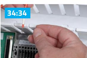
Assembler begins tagging each wire before connecting it to the terminal blocks.
