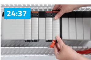
Finally, half of the process is complete and PLC Module is wired and snapped into place.
