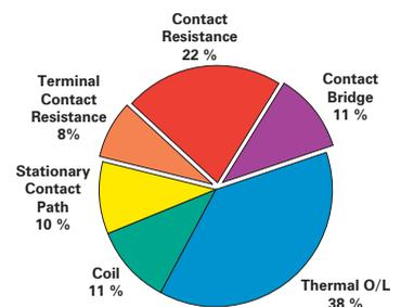
**Figure 4 - % Power loss within motor starter circuit.**
