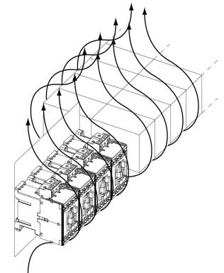
**Figure 3 - Convection along a row of devices can be interpreted as convection across a long horizontal bar.**
