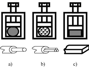
**Figure 2 - Typical wiring geometrics within wiring terminal.**
