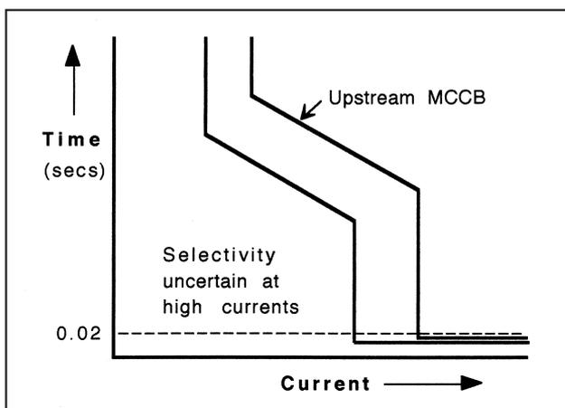
**MCCBs must trip quickly at high current levels.**
