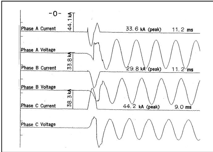
**Typical MCCB breaking 50 kA. Breaker starts to open very quickly and limits peak current.**
