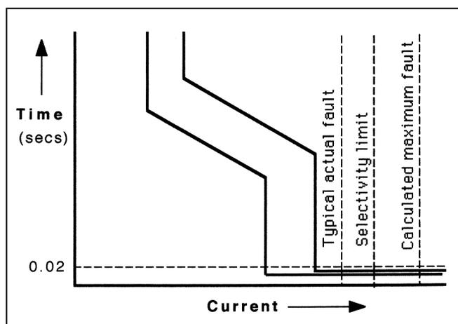
**Typical actual fault levels should be considered when designing for selectivity.**
