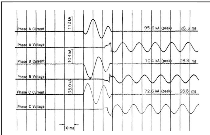
**Typical ACB breaking 50 kA. Breaker remains closed for 20 ms. (see delay in appearance of arc voltage)**
