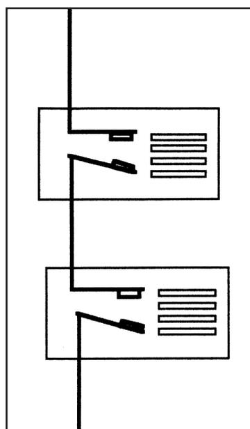
**A fault passing through two CBs can result in a high combined short circuit rating.**
