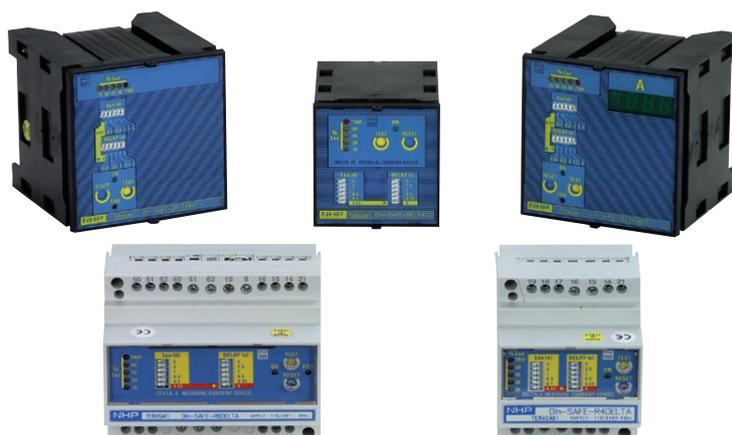
Phase and neutral conductors are passed through a toroidal transformer, creating a magnetic field proportional to its current. In normal situations the vector sum of the currents is zero even with unbalanced 3 phase loads.
