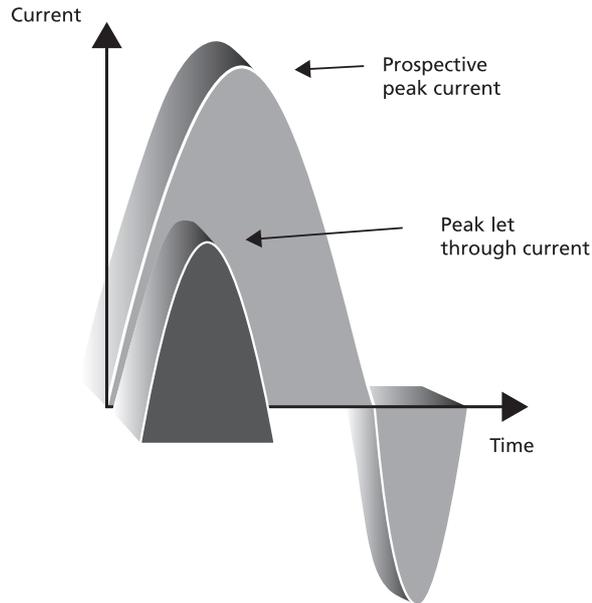
**Moulded case circuit breakers reduce both the peak current and duration of a short circuit**
