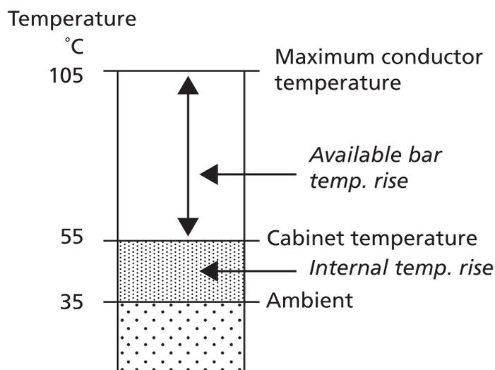
**Total cabinet temperature determines the available temperature rises on conductors.**
