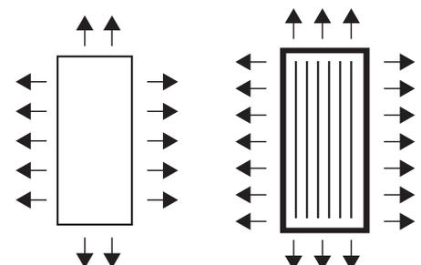
The emissivity of isolated flexible busbars is high than bare copper. Higher current ratings are possible.
