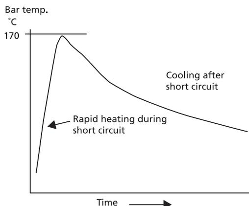
**Copper and insulating materials can withstand short term peak temperature.**
