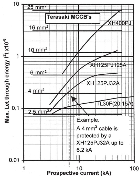
plotted on a circuit breaker time current curve. It can be seen from this that the circuit breaker will trip before the cable's maximum withstand has been reached.
