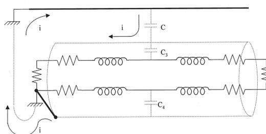
Figure 3. Screened Signal Conductors
