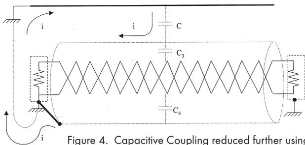
Figure 4. Capacitive Coupling reduced further using twisted pairs and shielding
