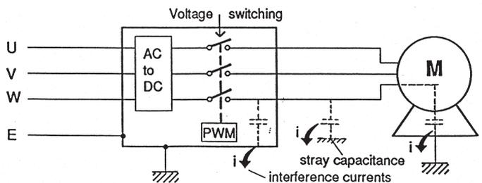
Figure 5. Noise Coupled Into the Earthing System
