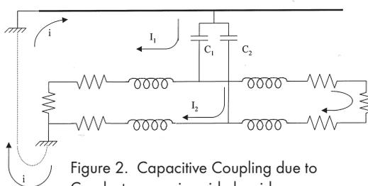
Figure 2. Capacitive Coupling due to Conductors running side by side
