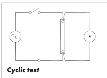
A common problem with connecting a stranded cable in a terminal is that movement of the cable can cause the strands to move and loosen the connection.
