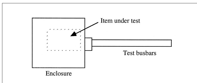
**Figure 4. Typical manufacturer's test for enclosed rating.**
