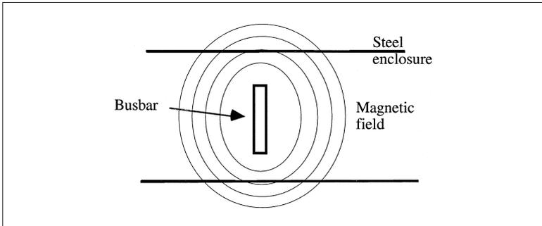
**Figure 3. Magnetic fields can cause severe eddy current heating of steel panels.**
