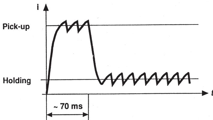
**Pick-up and hold-in current with electronic control**
