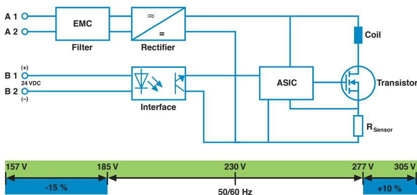
**The electronic circuit of the Sprecher + Schuh CA6 contactors allows a very wide operating voltage with precise opening and closing levels. The design includes EMC filters and a built-in PLC interface.**
