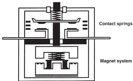
**Principle design of a contactor**
