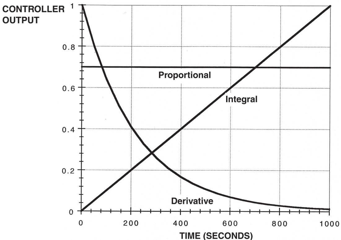
Figure 1. Controller output with step disturbance
