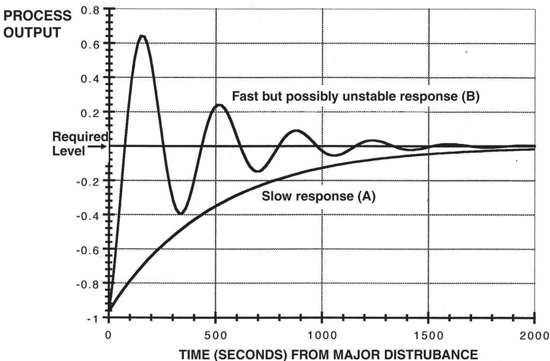
**Figure 2. Process output with step disturbance**
