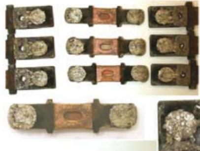
*Contactors' contacts: AC4 application after 20,000 operations*
