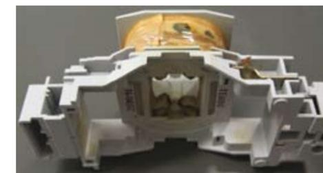
Failure due to excessive heat
