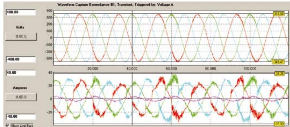
**surges** can have a dramatic impact on sensitive electrical equipment especially at the PCB level. Over voltages also affect insulation properties and when insulation fails, short circuits are likely.
