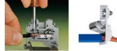
Each CAGE CLAMP® spring applies a pre-programmed force adapted for the specified cross-sectional wire type to a defined contact area. Once the CAGE CLAMP® is opened, a conductor can be inserted (illustrated above). A defined contact pressure presses the conductor into the surface of the current bar ensuring a gas tight, corrosion proof connection.
