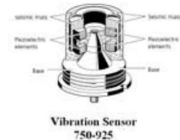
WAGO has developed a vibration monitoring system that overcomes many of the problems with existing vibration systems. The WAGO system consists of a vibration sensor that constantly measures both the mean value of the vibration severity and the 'shock pulse' value. Two such sensors can be monitored by the new WAGO vibration module 750-645.
