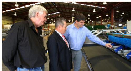
Using four cameras per lane, the InVision 9000 is able to view from the top and sides of the fruit covering 100% of the surface area of each piece of produce. With up to 60 images able to be captured while the fruit passes through the line, the accuracy achieved is extremely high, resulting in the separation of damaged fruit prior to shipping and the best return from the crops.
