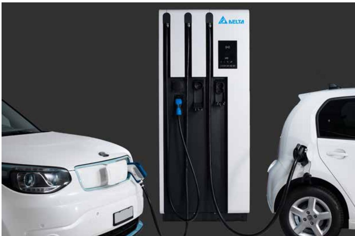
The Delta Ultrafast charger is a modular DC charger. The unit has up to a 150kW output that is reachable using 10kW DC modules. The base unit is 50kW, which would give a car an additional range of 200km to 300km. The Ultrafast charger provides the ability to upgrade to meet future charging demands. As standard, the Ultrafast charger comes equipped with CCS2 & CHAdeMO DC Plugs, and a Type 2 three phase AC plug that allows for charging at up to 43kW.
