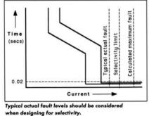
current ratings. Some circuit breakers act as current limiters and issue 30 provides great detail on how this is achieved and the benefits that result. The role of the breaker is to protect the downstream cable. Issue 32 discussed the three operating conditions under which this is required. Residual Current Devices are life saving devices and it is therefore important that they are installed correctly. This requires a good understanding of their purpose, what
