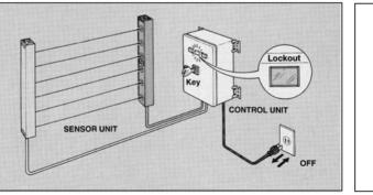
Light curtain. Presence sensing by electro-sensitive means.
