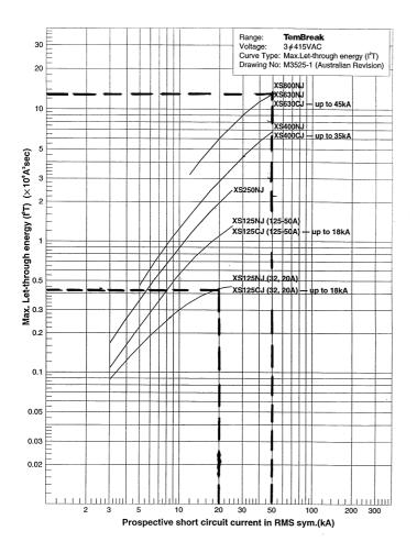
Fuses, on the other hand, have constant I<sup>2</sup>T values and these are usually given as two figures; 'pre-arcing' and 'total' at particular voltages.
