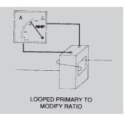
and they are mounted close together then no special selection is required. If the CT ratio is low (less than 200/5) and/or the cable run is long then the cable burden should be calculated and added to the burden of the connected device. The total burden should then be compared to the CT performance. It is common to quote the accuracy at different burdens and at low burdens it can be found that quite an inexpensive CT can have excellent accuracy.
