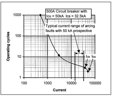
Circuit breakers can be selected on the basis of Icu. Actual fault currents are normally less than the circuit prospective.
