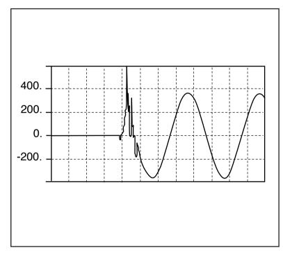
Transient voltage recorded during short circuit testing of a miniature circuit breaker. Actual peak is off scale.
