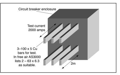
Typical test arrangement for enclosed current rating. Test busbars are of large cross section.
