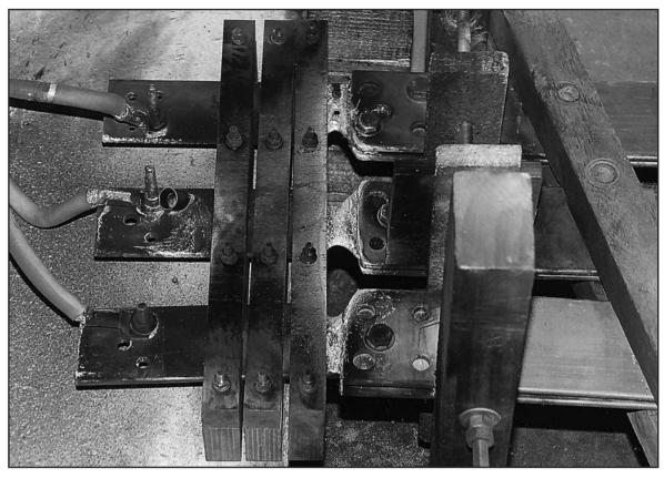
Flashover of test station terminals caused by a voltage transient. Test duration 0.2 seconds 50kA prospective current.
