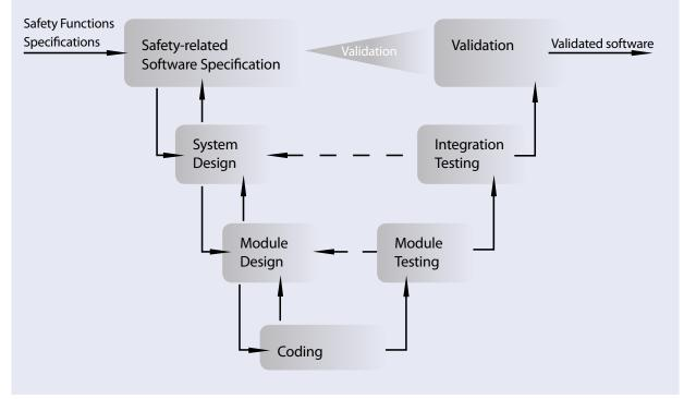
Figure 3 - Software Development Lifecycle used in ISO 13849-1
