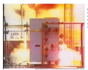
The adjacent picture is of a switchboard under test conditions being subjected to a short circuit.
