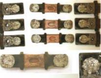
Contactor's contacts: AC4 application after 20,000 operations
