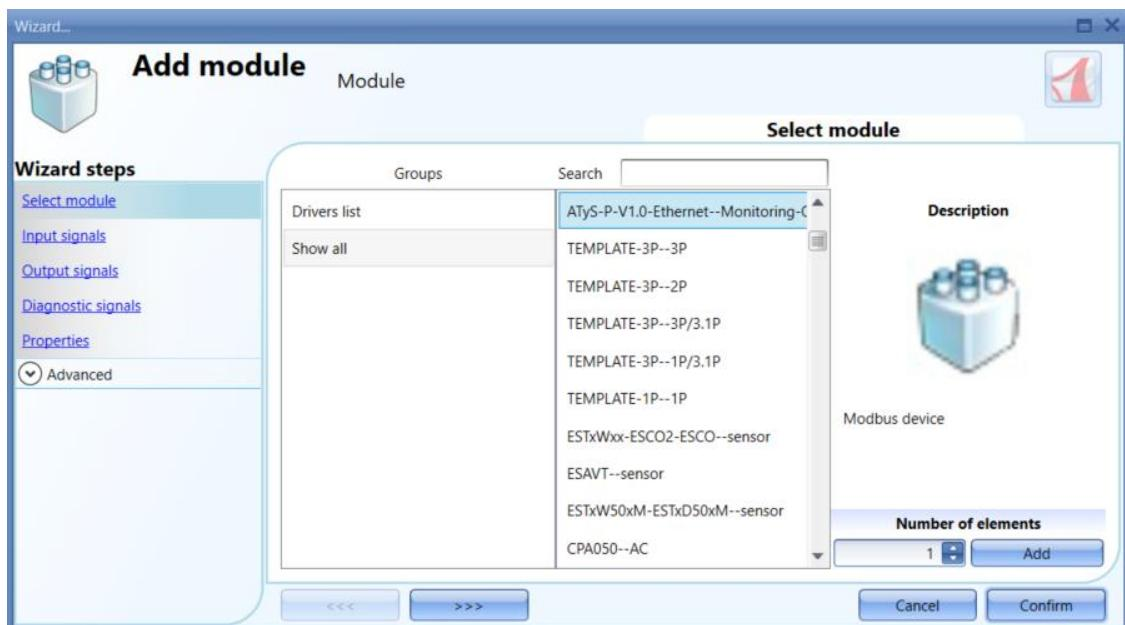
8. Before clicking on confirm go to properties and check the Modbus ID matches that of the ATyS p module (please refer to Annex I – 12. Communication menu – keypad navigation on page 99 of the ATyS p instruction manual for communication address and designation details). Click confirm.
