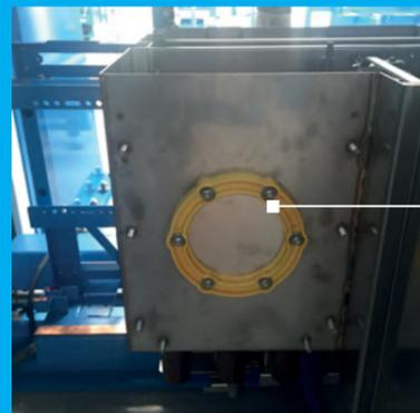
Pressure burst disc release system mounted at the bottom of the sealed tank
