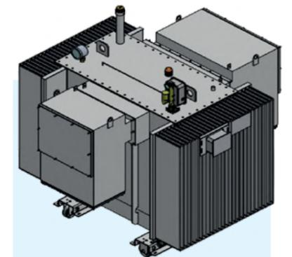
TES-OM -11- 0415-2000-Dyn11-K-H-M (kiosk style with HV plug-in bushings and LV flat busbar type bushing)
