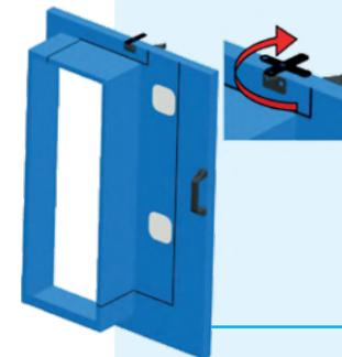
Access door to cable compartment. For safety, the door is mechanically interlocked whereby the earth switch must be closed before the door can be removed and the load break switch can't be closed with the door removed. The door can be padlocked to stop removal.
