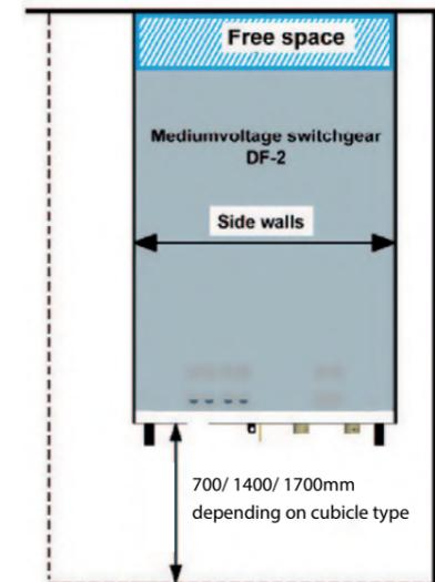
Side plates must be installed running to the wall to create an enclosed free space
