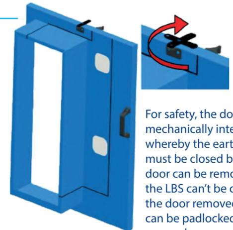
For safety, the door is mechanically interlocked whereby the earth switch must be closed before the door can be removed and the LBS can't be closed with the door removed. The door can be padlocked to stop removal.
