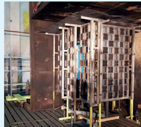
KEMA Labs testing of the DF2+ switchgear at 24kV
