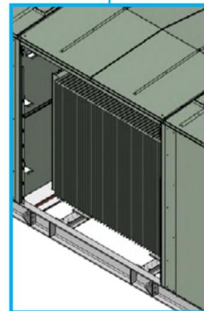
Transformer section is IP23D rated with both oil immersed or cast resin types
