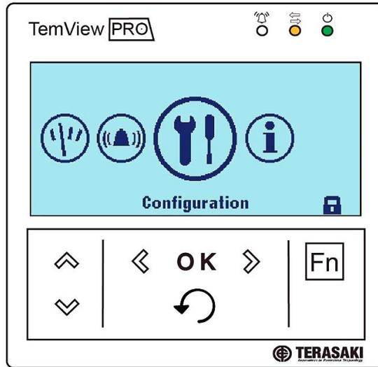
View and modify MCCB measurement and display settings, and reset of historical measurement data, alarms and events.
