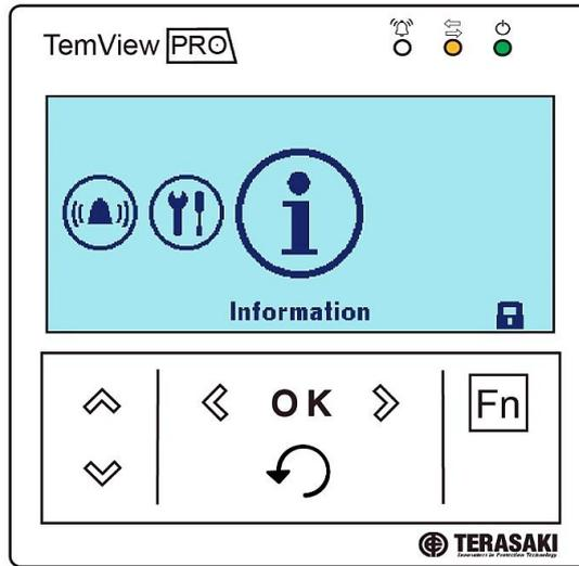
View the status and identification information of the MCCB and historic trip and alarm logs include SMART Auxiliary counters.
