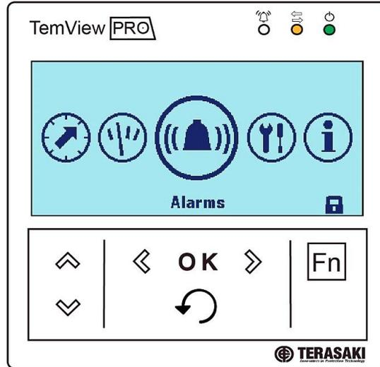
View and modify alarms for various types of events based on system status and live monitoring of parameters, including custom alarms, PTA and Optional Alarm (OAC) contacts.
