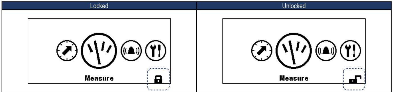
To unlock the TPED, press the Function Key “Fn” and enter the password by increasing or decreasing each of the four digits to the required value.
