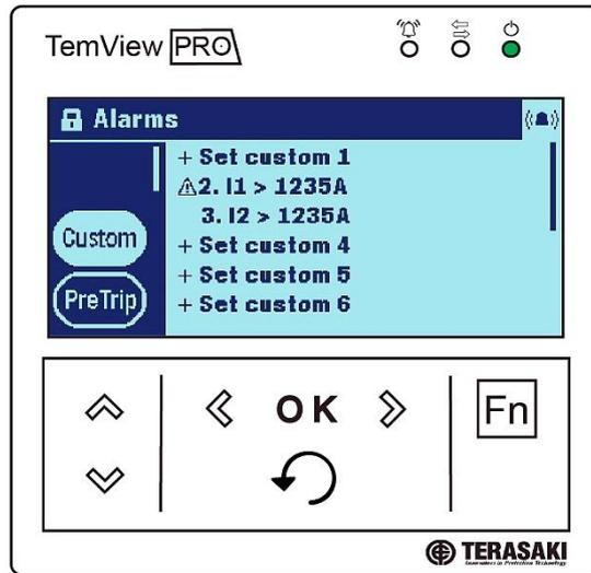
Custom alarms make it possible to produce alarms based specific events and measurements made by the P\_SE OCR. They are only available to be configured and displayed using the TPED and/or TPCM in conjunction with the P\_SE MCCB.
