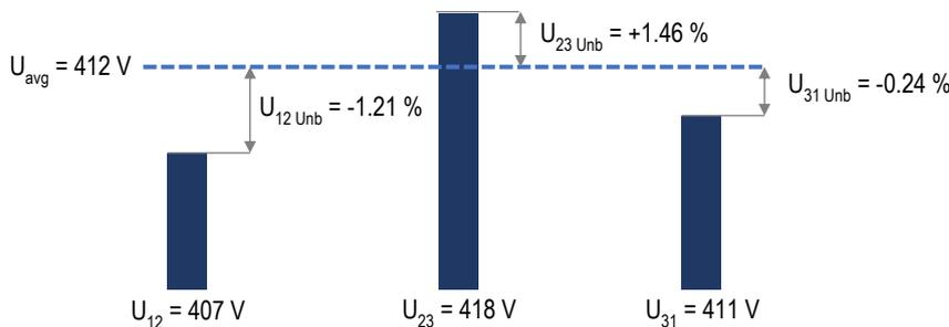
$$U_{\text{avg}} = \frac{U_{12} + U_{23} + U_{31}}{3} = \frac{407 \text{ V} + 418 \text{ V} + 411 \text{ V}}{3} = 412 \text{ V}$$
