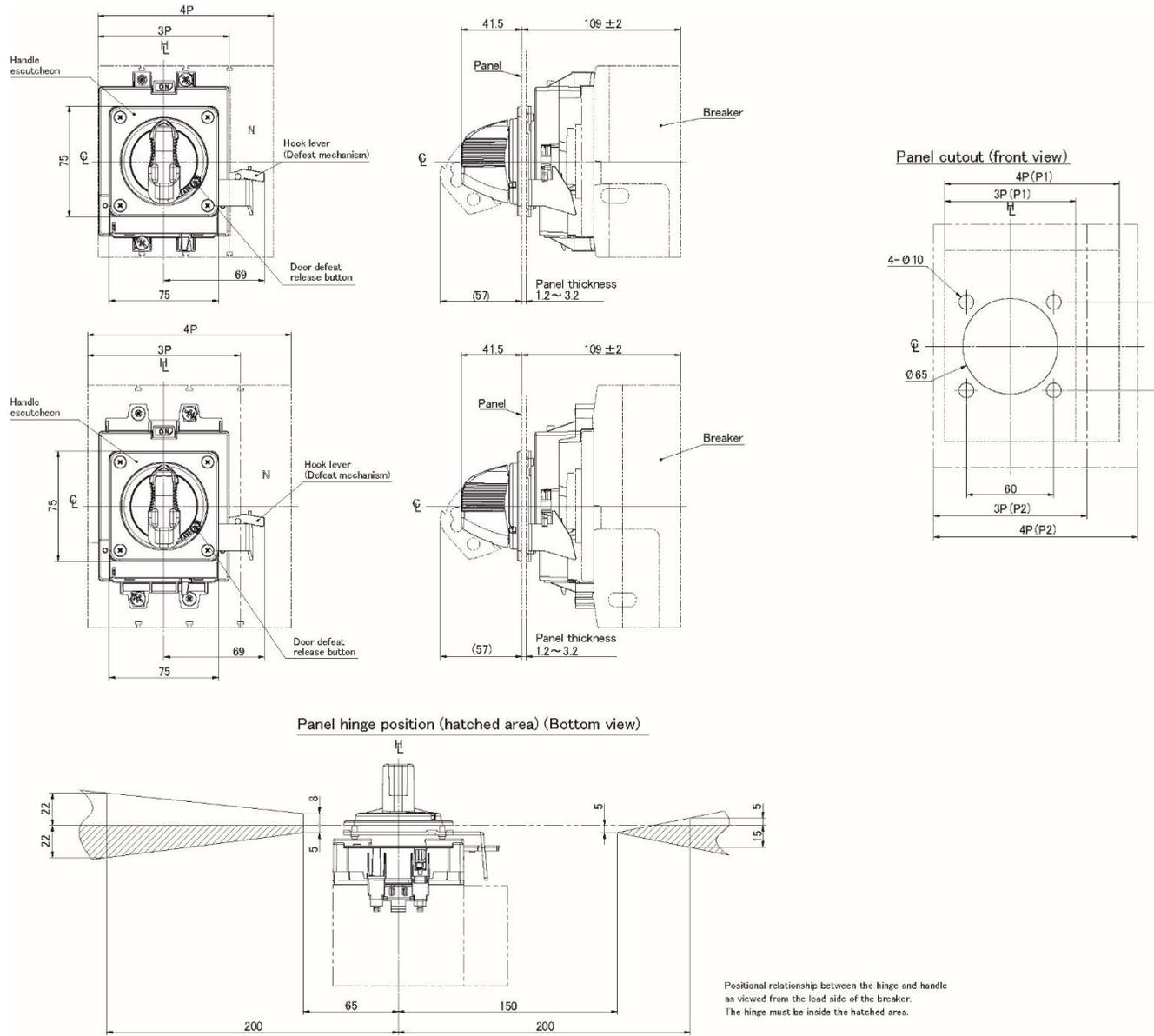
Positional relationship between the hinge and handle as viewed from the load side of the breaker. The hinge must be inside the hatched area.
