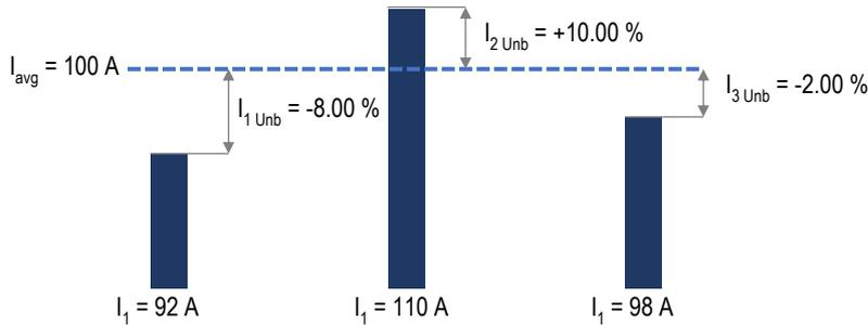
$$I_{\text{avg}} = \frac{I_1 + I_2 + I_3}{3} = \frac{92 \text{ A} + 110 \text{ A} + 98 \text{ A}}{3} = 100 \text{ A}$$
