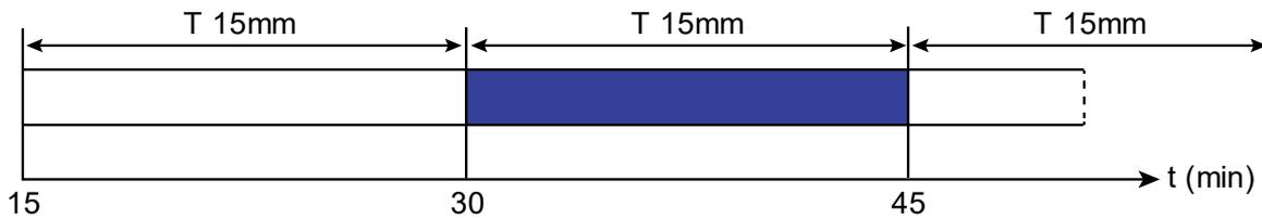
The duration of interval T can be configured between 5 and 60 minutes in increments of 1 minute.
