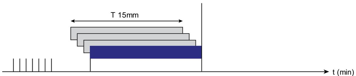
The duration of interval T can be configured between 5 and 60 minutes in increments of 1 minute.
