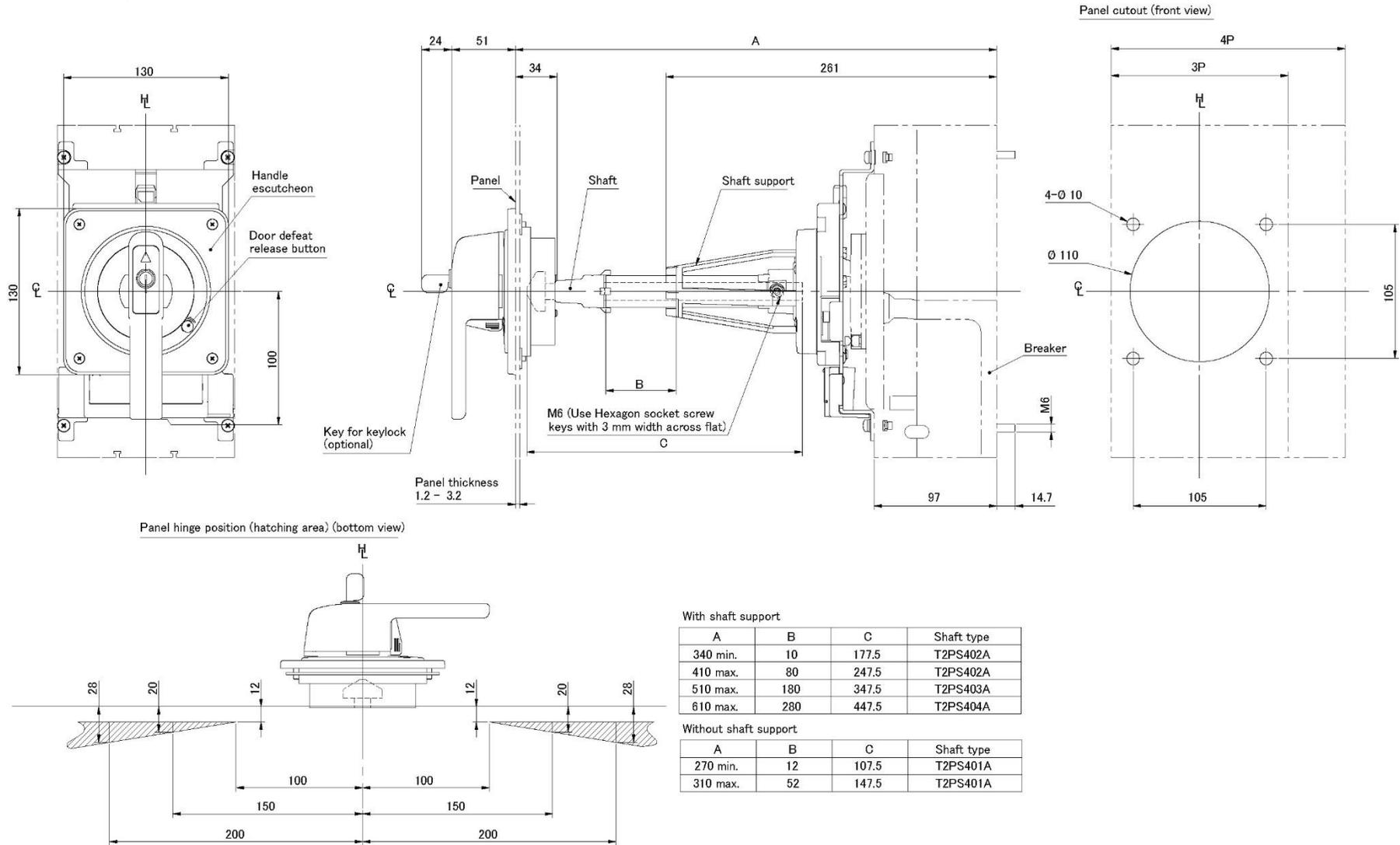
Positional relationship between the hinge and handle as viewed from the load side of the breaker.
