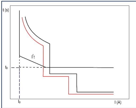
Adjustments to the  $I^2t$  for GF setting can be made using one or a combination of the below methods:
