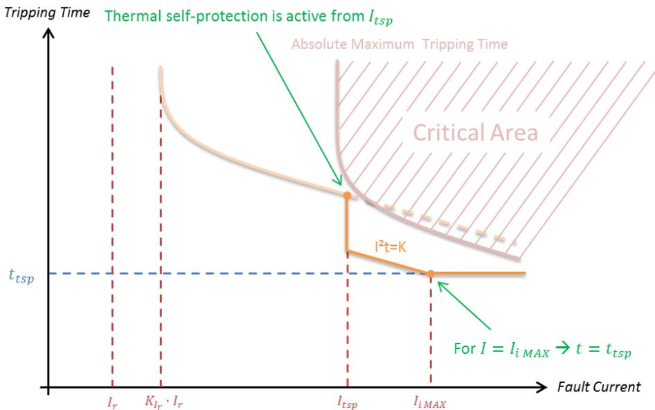
Thermal self-protection is only on the following MCCBs. When activated,  $I_{tsp}$  and  $t_{tsp}$  values are specified as follows:
