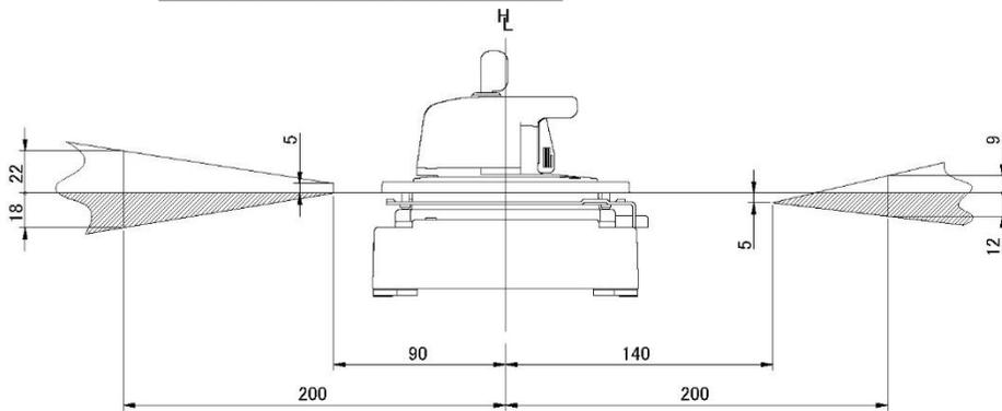
Positional relationship between the hinge and handle as viewed from the load side of the breaker.
