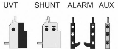
**Notice:** Only 2 internal accessories can be mounted on the right-hand side of a P400 and P630 MCCB. Under no circumstances can 3 or more be installed.
