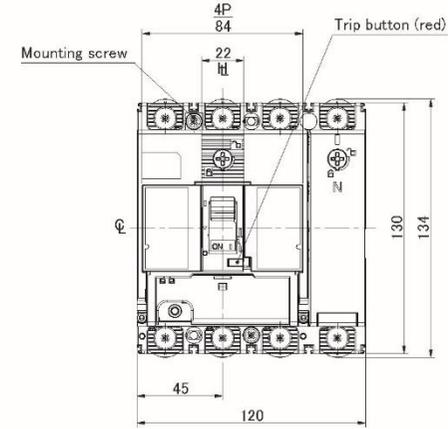
Drilling plan (top view)
