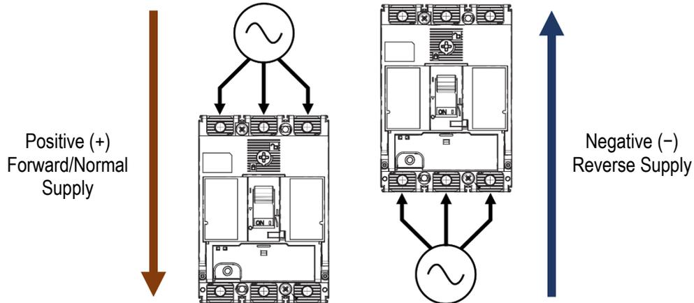
Changes to the power flow direction can be made using one or a combination of the below methods:
