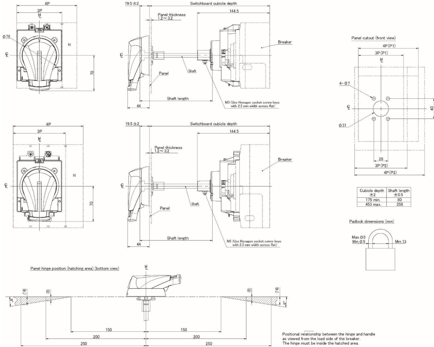
Positional relationship between the hinge and handle as viewed from the load side of the breaker. The hinge must be inside the hatched area.
