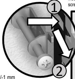
Insert the 4 door mounting screws in the designated slot
