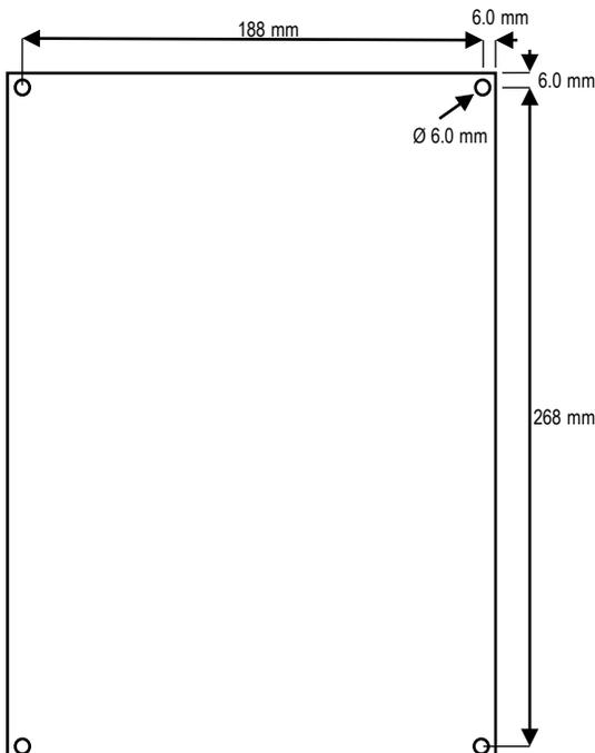
Installer to select appropriate fasteners to suit size 6mm mounting holes of unit to mounting material
