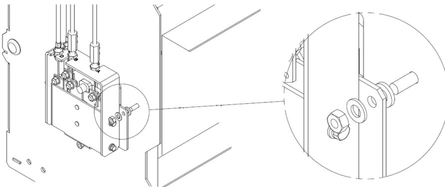
22. Push the third spacer between the carriage side plate and the mechanical interlock mechanism so it lines up with the empty third mounting hole. From The outside of the carriage, screw in the M6 x12mm bolt to secure as shown below. Repeat step 22 for ACB 2.
