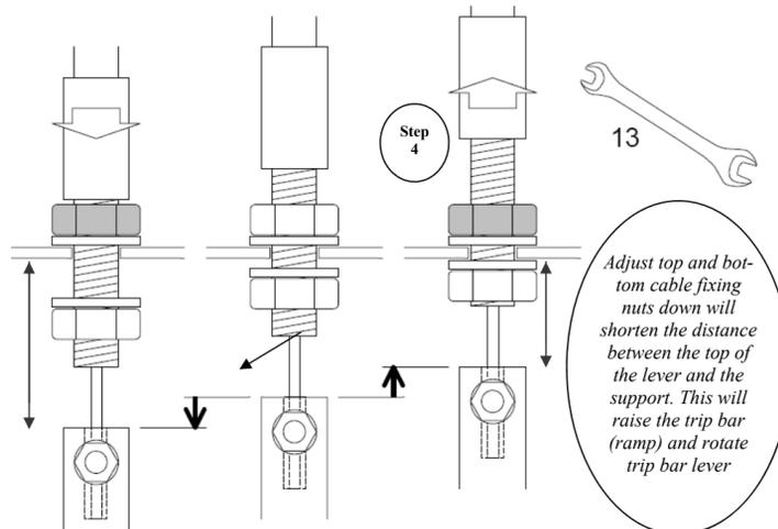
5. With the play now removed, try to insert, but do not force jig 2 in between the trip bar and the trip bar lever of ACB 1 as shown below. Because the play has been removed it should not be possible to fully insert jig 2 with minimal force.
