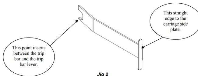
6. Slightly lengthen the inner core to allow full insertion of Jig 2. Do this by moving the ACB 1, port A top and bottom fixing nuts 'up'. Adjust the fixing nuts ONLY until Jig 2 can be fully inserted with minimal force as shown below.
