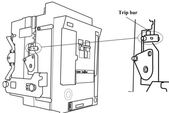
The **trip bar** is moved via the **trip bar lever** which is located on the **mechanical interlock mechanism**. The **trip bar lever** looks like a **ramp**.
