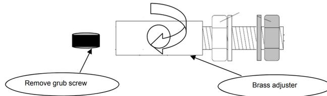
5. Insert the 'open' end of the cable into the brass adjuster. Observe through the grub screw hole that the black outer sheath of the cable is fully pushed into the brass adapter. The inner core should protrude at least 45mm from the ends of the black outer sheath on both 'open' and 'fixed' cable ends (in other words the total inner core length should be at least 90mm longer than black outer sheath total length after the loose brass adjustment end is fitted).
