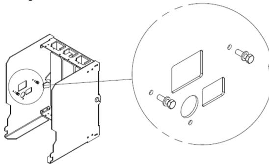
10. Attach the **Jig 1** to both **carriage interlock mechanisms**. The lever protrusions on the carriage interlock mechanisms will with some manual manipulation line up and slot into the cutouts on **jig 1**. Secure with the **three 12mm M6 pan head screws** as shown below.
