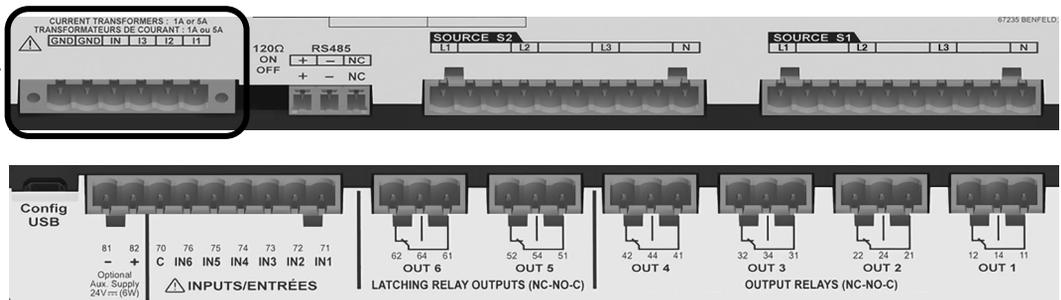
\*use when current sensing is required for current, power and energy measures on the C65 (1A or 5A CTs)
