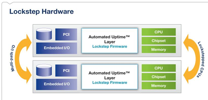
The Automated Uptime Layer detects, isolates and resolves faults before they cause downtime.
