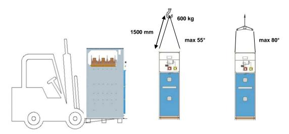
In order to safely and securely lift the unit, use the provided **lifting eyebolts**. Secure the slings or rocker arms tightly to all four lifting eyebolts before moving the unit into its final position.
