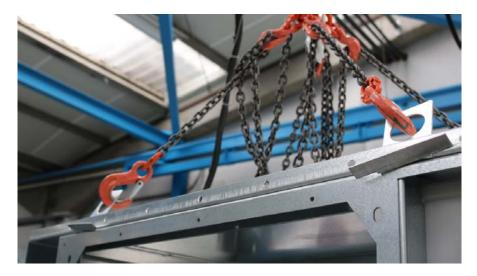
Version B: lifting eyebolts are secured using bolts:
