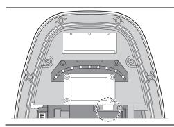
Insert the SIM card into the socket and ensure the connection is well connected.
