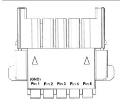
4. Connect the signal cable according to pin definition\* and must connect to the ground(Pin 1).
