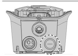
1. Remove the water proof cap and pass through the Ethernet cable with appropriate conduit or cable gland.
