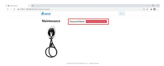
3. Confirm if the user want to reset the password. After clicking the button "Yes", the EVSE will restart automatically.
