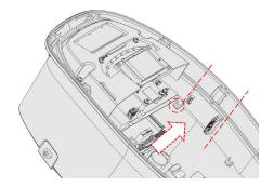
1. Based on the tenon, attach the connector to the inner surface of EVSE along the edge.
