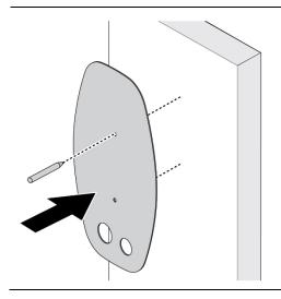
The EVSE is a stationary wall-mounted equipment. Using the template to mark the screw locations for the mounting bracket and cable holder (optional).
