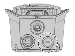
3. Remove the water proof cap and pass through the signal cable with appropriate conduit or cable gland.
