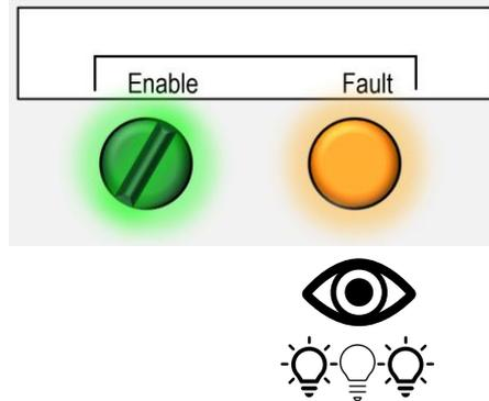
**Example –** The *Fault* indicator flashes once every 2 seconds at a 50% duty cycle, with a 2 second pause between flashing sequences, corresponding with Fault code '2' – with 2x flashes per sequence:
