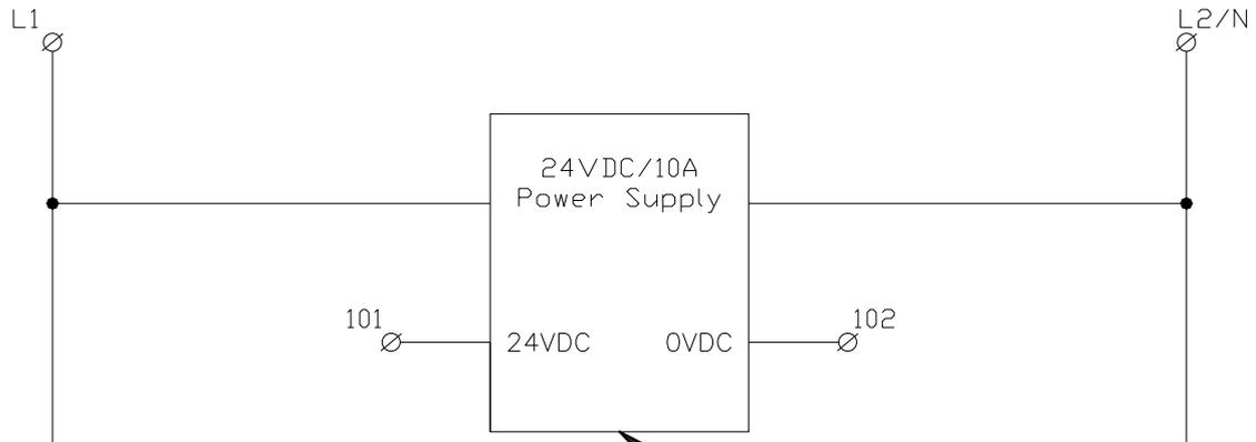
PSU locate as close as possible to iRRD, or calculate appropriate conductor size based on distance to iRRD and peak current.
