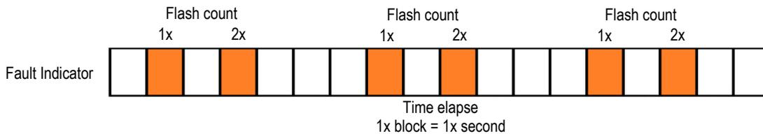
The *Fault* indicator will continue to flash the fault code and prevent any further commands to be issued to the TemRack *iR*. To reset the fault, either cycle the *Enable* switch OFF and ON, or cycle the power supply to the TemRack *iR*.
