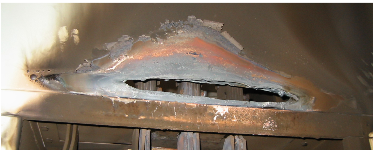
Above Result of switchboard arcing faults
