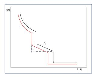
The below graphic illustrates the difference between  $I^2t$  enabled and disabled with a  $I^2t$  curve based on  $I_r = 630A$  for reference.
