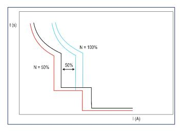
The Neutral Coefficient percentage can be adjusted from the N (%) dial. GF protection is also turned ON or OFF by setting the dial to any position on the right for ON, or any position on the left for OFF. See <u>Ground/Earth Fault Protection (GF)</u> section for more information on the N (%) dial.
