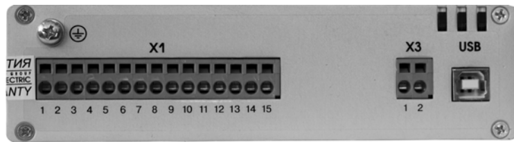
Figure 71 Terminal arrangement of the the CM
