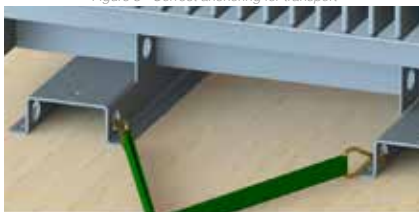
Figure 3 - Correct anchoring for transport
