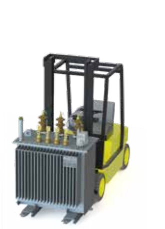
Figure 5 - Lifting using a lift truck
